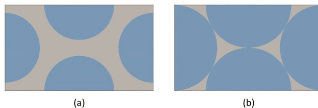
Fig. 6 Unit cells \mathcal{U} for hexagonal suspensions of monodisperse liquid 2-spherical inclusions of radius A at volume fractions (a) c = 0.6 and (b) c = 0.905 .
